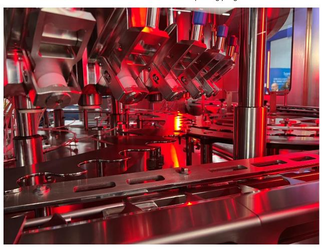
> ZACMI filling machine in clean design with full CIP option and innovative filling technologies.
