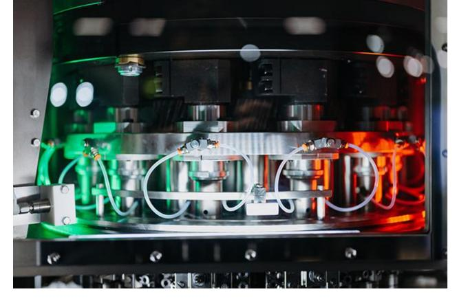
> There were insights into the fully automatic and temperature-monitored dual-circuit oil circulation lubrication of the new Zacmi can sealing machine.
